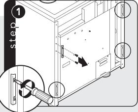
Unscrew four standoff brackets and remove.
